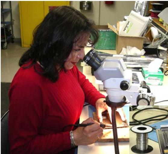
Mary Ellen builds the boards, using a microscope, solder paste, sometimes tweezers. She receives the “picture” of what the finished board should look like, the parts and the parts list from the
